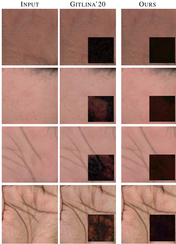
Figure 10: Antera device comparisons. Our reconstructions consistently exhibit less errors than in the previous work. From top to bottom the mean square error ([GGD*20] vs. ours) is: (0.0142 \text{ vs. } 1.65 \cdot 10^{-6}) ; (0.1016 \text{ vs. } 2.31 \cdot 10^{-5}) ; (0.0585 \text{ vs. } 1.08 \cdot 10^{-5}) ; and (0.2239 \text{ vs. } 8.93 \cdot 10^{-5}) .
