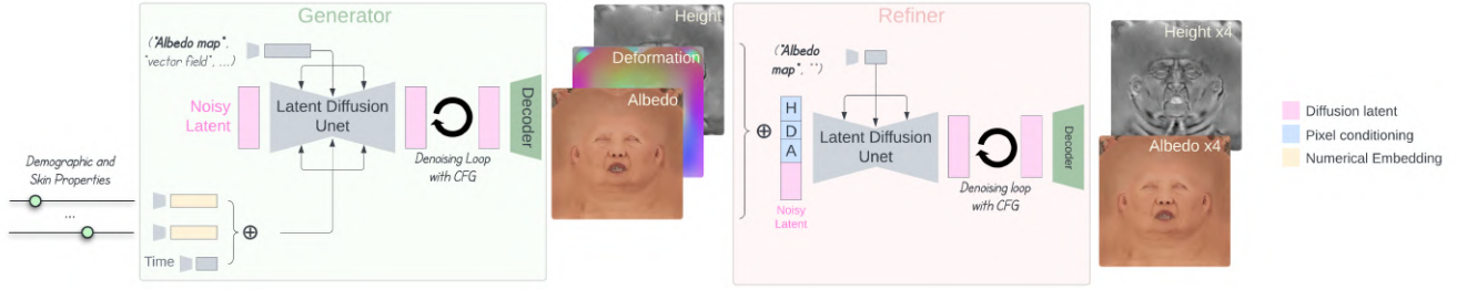
Figure 2: Overview. Our model generates a deformation texture D , a height map H , or an albedo map A at mid resolution depending on a text prompt \mathbf{p}_G and controlled by various conditions. Then, a Refiner receives the concatenation of these three maps to upsample the map specified by another prompt \mathbf{p}_R by \times 4 resolution.
